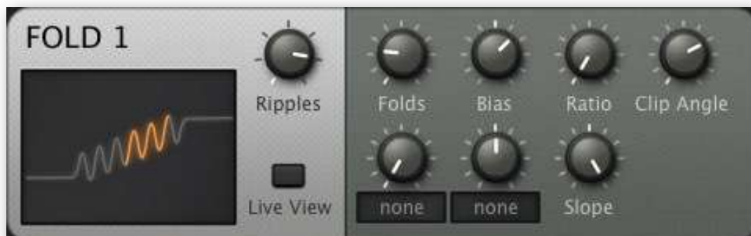
Fold module panel with 6 Ripples, 22% Folds, 30% Bias and maximum Slope
