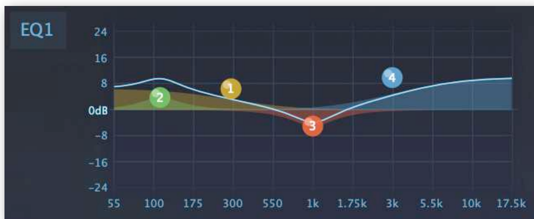
Equalizer module, bass+treble boost, dip around 1 kHz
