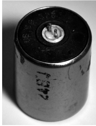
Figure 2.12 An SM-24 geophone with a diameter of about 30 mm.
